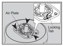
3. Remove air plate and filter.
