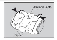
2.Slide the old or worn balloon cloth over the top of the lamp guard assembly.
