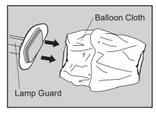
3. Slide the new balloon cloth over the top of the lamp guard assembly.
