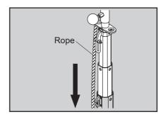
⚠DANGER When lowering down the mast please pull the rope vertically to prevent the lighting system from overturning.
