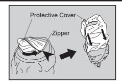
6.Store the power cable inside the pocket of the protective cover. Zip up the protective cover and loop fastner at the bottom of the protective cover.
