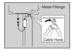
5.Bind the noise filter of power cable on the 3rd mast with cable tie.
