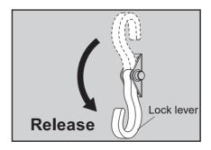
2.Pull the rope downward vertically untill to the desired height. Apply the lock lever to lock on the mast.
