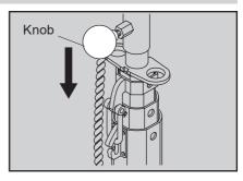
2.Release the safe stopper from the lock-hook.
