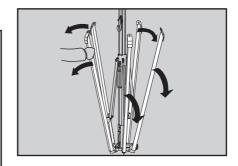
4. The latch will be set at top hook (Position 0) when the pentapod is deployed. Do not use it while it is set at top hook.
