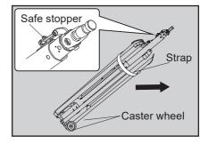
2. Squeeze both tabs on each side of buckle to unlock strap and allow pentapod legs to be deployed.
