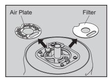
4.Install a new filter and reinstall an air plate.
