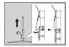
3. Grab one of the legs. Pull upward until all legs are fully retracted and are in the stow position. Place the strap around all 5 legs.
