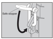
4.Disconnect the connector. Remove the cable hook of the AC power cable from the metal fittings located on the bottom plate of the light assembly.
