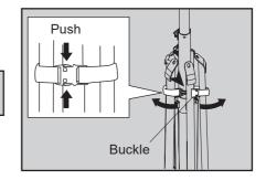
3.Pull upward on the mast and let the pentapod legs deploy.
