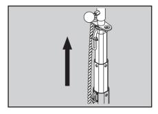
4. The mast will stop rising by applying the lock lever at the desired height.
