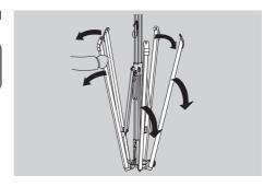
4.The latch will be set at top hook (Position 0) when the pentapod is deployed. Do not use it while it is set at top hook.
